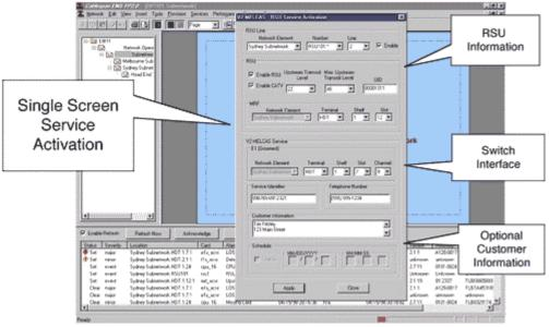
The next step after completing configuration and provisioning of the RSU and its supporting MRF is to activate customer service. *Figure 6* shows a single screen
