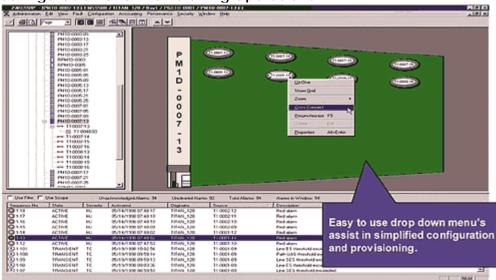
Figure 4. Use of Graphics and Drop-Down Menus to Simplify Configuration and Provisioning Operations
