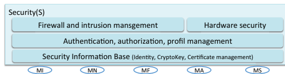
Fig. 9: Security layer of the ITS-Station communication architecture
