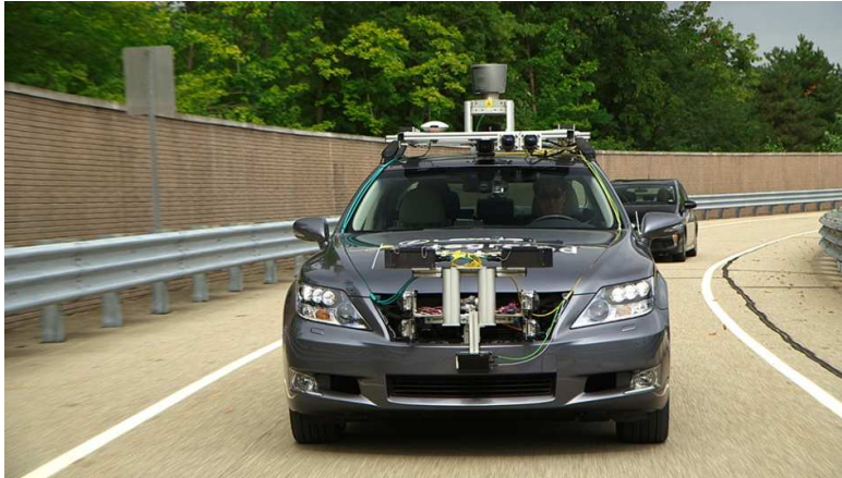
Figure 8.15. V2V based Cooperative-adaptive Cruise Control test vehicle. (Source: Toyota)
