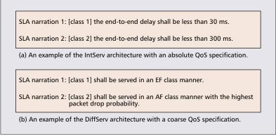
**Figure 3.** Example differences, in terms of the SLA policy, of IP QoS architectures.
