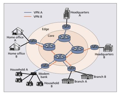
**Figure 1**. *The general IP-based VPN architecture.*
