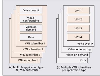
Figure 2. Two examples of how VPN SPs deliver QoS.
