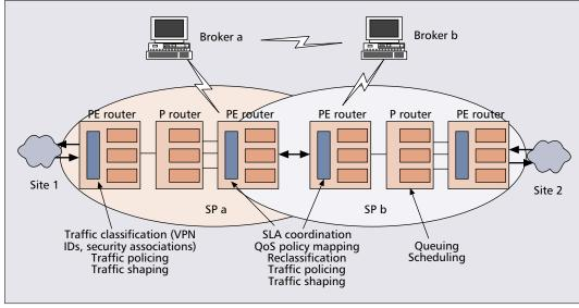
Figure 6. The VPN data flow across multiple SP domains between sites 1 and 2.
