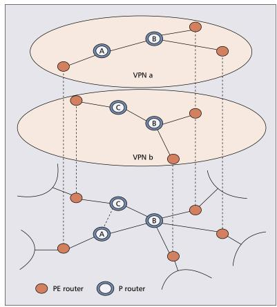
**Figure 5.** An example of VPN resource provisioning, where QoS-warrant routes (topologies) of VPNs a and b have been reserved from the original network.
