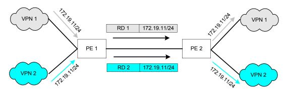
The Route Distinguisher is a way to make the VPN addresses unique, but does not give any information about the route, such as identifying the VPN. Instead, the VPN to which the route belongs is carried in a separate BGP attribute – a Route Target Extended Community. This allows a PE router receiving a VPN-IPv4 route to install the route in the correct forwarding table.
