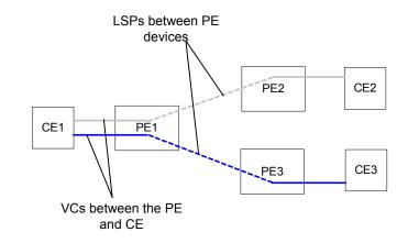
This is a relatively straightforward approach, and MPLS traffic engineering can be used to provide quality of service if this is required by the customer. However, it does not scale well in the provider network for the following reasons.
