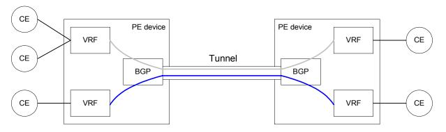
One worry that customers may have with a VPN is that the provider may accidentally make a mistake with the VPN configuration. Having a competitor's customer site join your network is likely to be viewed as a bad thing! Although it is difficult to prevent configuration errors, it is some comfort if you can spot this type of error, and **draft-ietf-ppvpn-l3vpn-auth** offers a means for CE devices in layer 3 VPNs to check that the other CE devices in the same VPN are allowed to be there.
