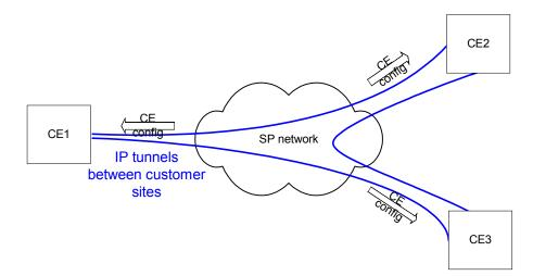
There are a couple of Internet drafts describing how the provider can manage the CE devices remotely. These describe ways in which configuration information can be transmitted by the service provider to the CE-devices for layer 2 VPNs (see **draft-lee-ce-based-vpl**), and layer 3 VPNs (**draft-ietf-ppvpn-ce-based**).
