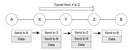
This tunneling of data means that the P devices do not need to be aware of the VPNs, but just need to be able to forward tunneled data. This is important as it reduces the network resources consumed by the VPN and the amount of configuration required to set it up.
