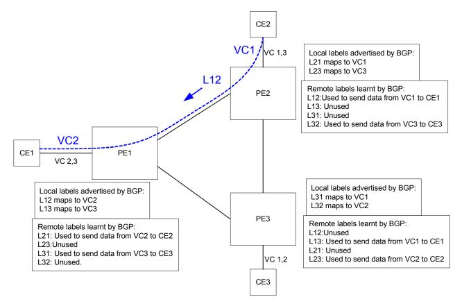
The next step is to set up the connections (typically ATM or Frame Relay Virtual Circuits) between the CE devices and the PE devices. Each CE is configured with a separate VC for each remote CE device that it wishes to connect to. These VCs are typically chosen so that there is a simple algorithm mapping from the remote CE identifier to the identifier of the VC to use.
