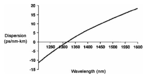
Figure 11. Typical Dispersion vs. Wavelength Curve
