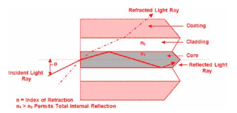
A protective coating is applied to the glass fiber as the final step in the manufacturing process. This coating protects the glass from dust and scratches that can affect fiber strength. This protective coating can be comprised of two layers: a soft inner layer that cushions the fiber and allows the coating to be stripped from the glass mechanically and a harder outer layer that protects the fiber during handling, particularly the cabling, installation, and termination processes.
