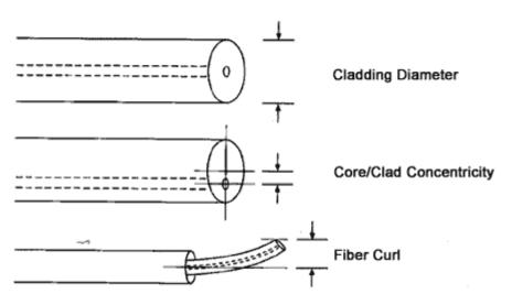
Figure 8. Cladding Diameter, Core/Clad Concentricity, and Fiber Curl
