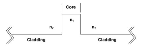
Figure 6. Index Profile of a Matched-Clad Fiber Design
