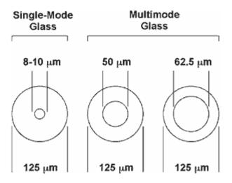
Figure 3. Optical Fiber Sizes
