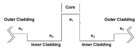
Depressed-clad fibers are made with two different cladding glasses that form an inner and an outer cladding region. The inner cladding region adjacent to the fiber core has an index of refraction that is lower than that of pure silica, while the outer cladding has an index equal to that of pure silica. Hence, the index of the glass adjacent to the core is depressed.
