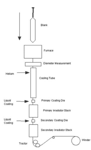
Figure 5. Optical Fiber Drawing Process
