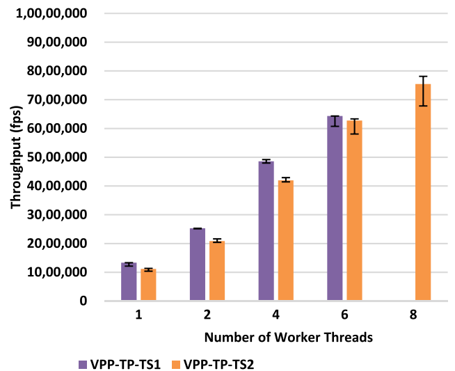
(b) the CPU frequency was set to 1.2 GHz at TS1 and 0.8 GHz at TS2 (The results with 6 workers on TS1 and with 8 workers on TS2 are limited by the Tester performance.)
