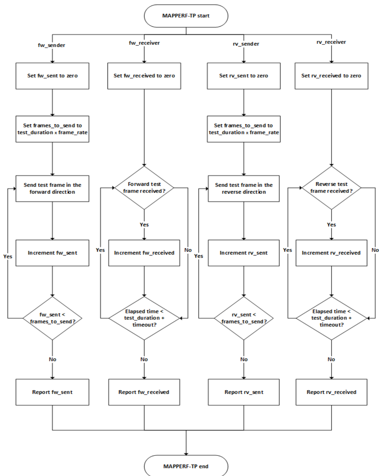
FIGURE 16. The Basic Flowchart of Mapperf-tp.
