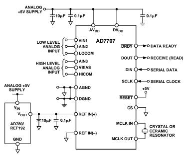
Figure 10. Basic Connection Diagram for 5 V Operation
