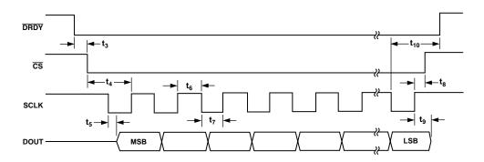
Figure 18. Read Cycle Timing Diagram
