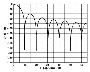
Figure 14. Frequency Response of AD7707 Filter
