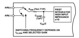
Figure 12. Unbuffered Analog Input Structure
