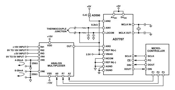
Figure 24. Data Acquisition System Using the AD7707
