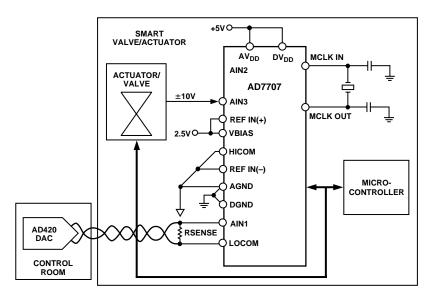
Figure 25. Smart Valve/Actuator Control Using the AD7707
