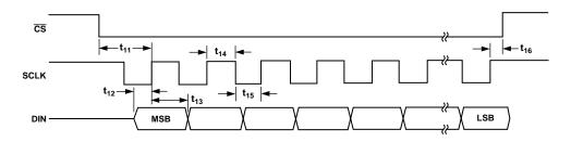
Figure 19. Write Cycle Timing Diagram
