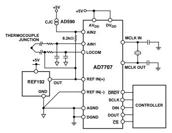
Figure 28. Thermocouple Measurement Using the AD7707
