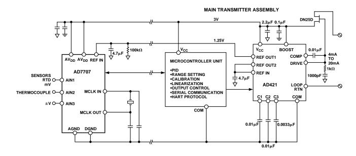
Figure 26. Smart Transmitter Using the AD7707
