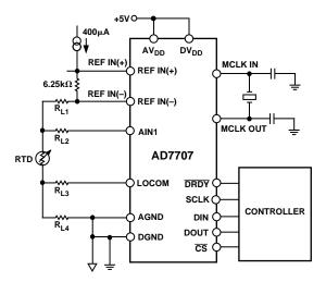
Figure 29. RTD Measurement Using the AD7707
