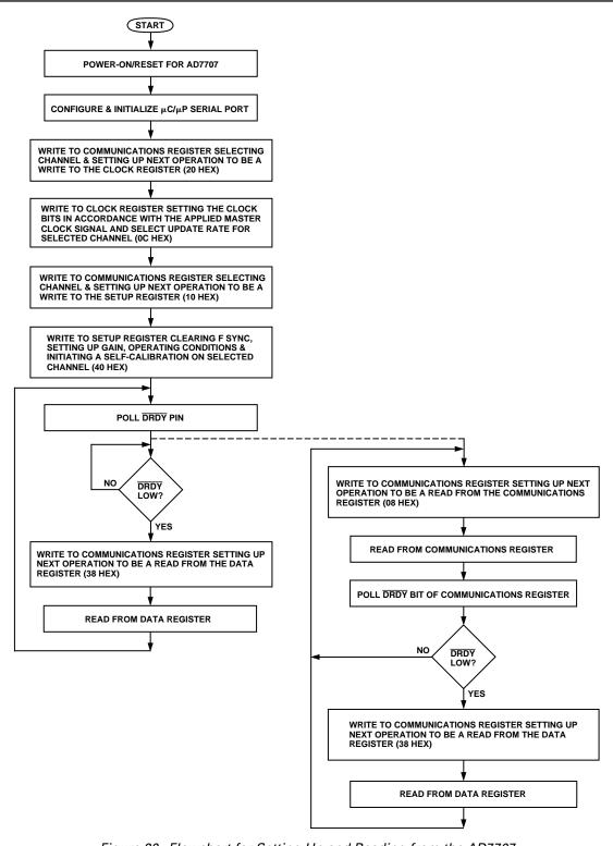
Figure 20. Flowchart for Setting Up and Reading from the AD7707
