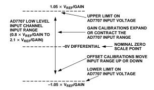
Figure 15. Span and Offset Limits for Low Level Input Channels AIN1 and AIN2
