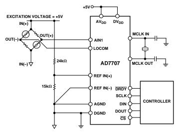
Figure 27. Pressure Measurement Using the AD7707
