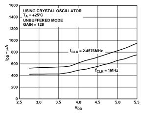
Figure 17. I<sub>DD</sub> vs. Supply Voltage
