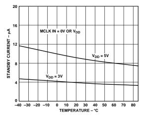
Figure 9. Standby Current vs. Temperature
