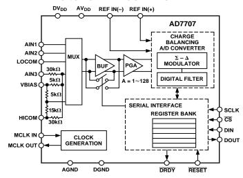
The AD7707 is ideal for use in smart, microcontroller or DSP-based systems. It features a serial interface that can be configured for three-wire operation. Gain settings, signal polarity and update rate selection can be configured in software using the input serial port. The part contains self-calibration and system calibration options to eliminate gain and offset errors on the part itself or in the system.
