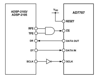
Figure 23. AD7707 to ADSP-2103/ADSP-2105 Interface
