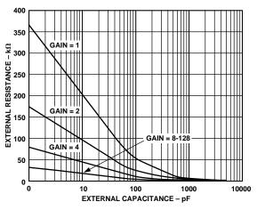
Figure 13. External R, C Combination for No 16-Bit Gain Error on Low Level Input Channels (Unbuffered Mode Only)
