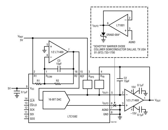
Figure 2. Driving I<sub>OUT2</sub> from AGND with a Force/Sense Amplifier
