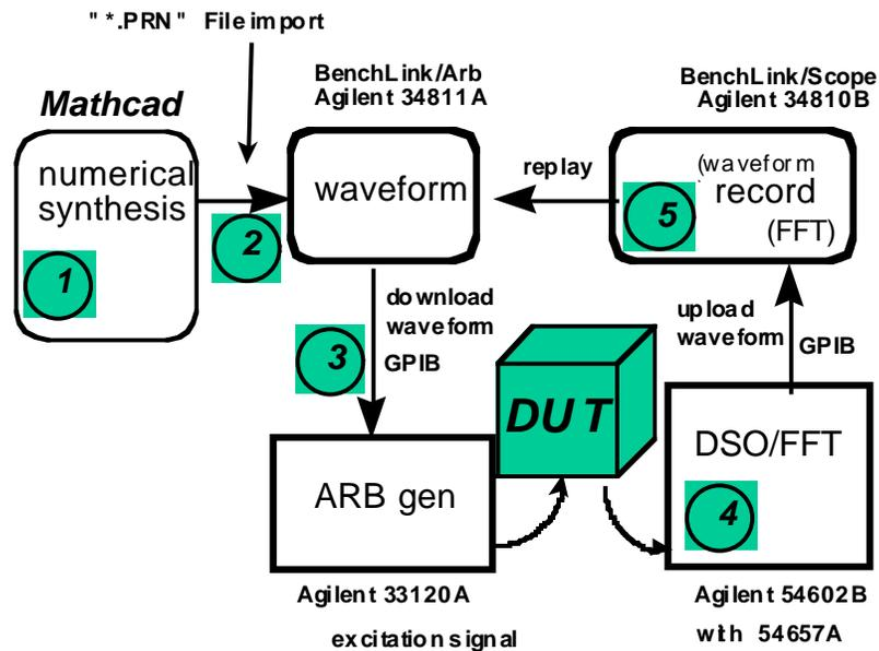
Fig. 1: Setup of experiment
