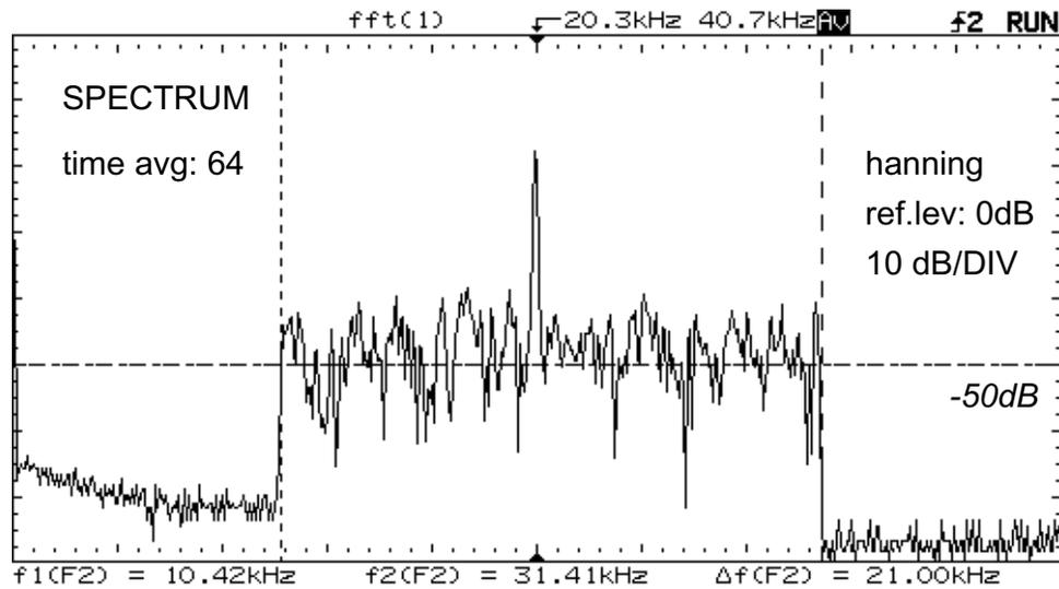
Fig. 5: Generate waveform at 10.1 Hz base arb. frequency, and measure the spectrum of live "signal + noise"
