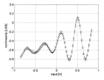
Fig. 3. FFT-test results for the first simulated ADC, reporting the true INL (---) and the estimated one for the 8-bit (000), 12-bit (xxx), 16-bit (+ + +), and 20-bit (\* \* \*) case.
