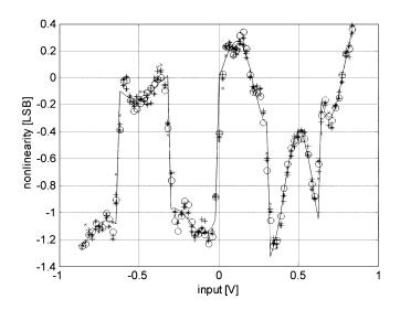
Fig. 5. FFT-test results for the third simulated ADC, reporting the true INL (---) and the estimated one for the 8-bit (000), 12-bit (xxx), 16-bit (+++), and 20-bit (\* \* \*) case.
