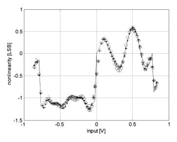
Fig. 4. FFT-test results for the second simulated ADC, reporting the true INL (---) and the estimated one for the 8-bit (000), 12-bit (xxx), 16-bit (+ + +), and 20-bit (\* \* \*) case.
