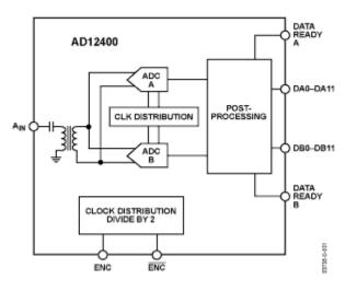
The <u>AD12400</u> comprises *two* high-speed AD9430s, and leverages time *interleaving* and AFB (advanced post-processing technique - *Advanced Filter Bank*) to attain a high level of performance
