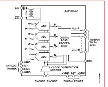
The <u>AD10678</u> integrates *four* AD6645s, a clock distribution system, and a complex programmable logic device (CPLD) that has been configured to provide a high-speed *addition* algorithm
