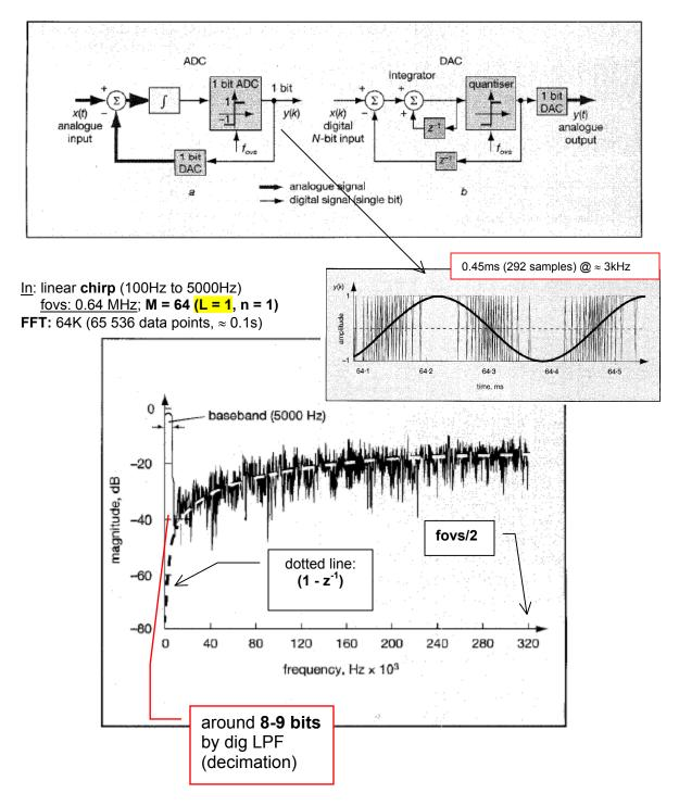
A second-order estimate of e[n] may be formed by assuming that the error e[n] varies <u>linearly</u> with time. In this case, an *estimate* of the current error e[n] may be computed by changing the previous error e[n-1] by an amount equal to the change between e[n-2] and e[n-1]. The second order *error* estimate is thus
