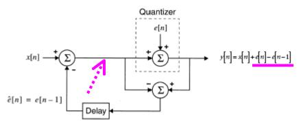
With a few straightforward steps, the system can be transformed into that of Fig below, where the delay element is now immersed in an integrator feedback loop.
