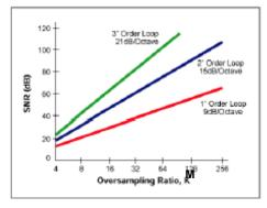
Relationship between order of sigma-delta modulator and the amount of oversampling necessary to achieve a particular SNR
