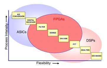
As a result, FPGAs have significantly invaded the application task space as shown by the center bubble in the task diagram above.
