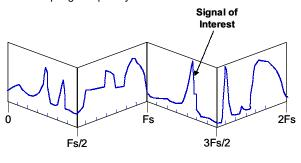
The third sampling mode, called undersampling or sub-sampling, is ideal for many systems that use an analog RF translator front end. These receivers usually deliver IF outputs, often at 21.4 or 70 MHz, with bandwidths ranging from a few kilohertz to tens of MHz, depending on the receiver.
