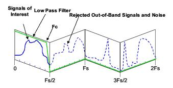
For the baseband **wideband** sampling mode, where we want to look at everything from DC up to a frequency below the half sampling rate, we can install a low pass filter with a cutoff frequency, Fc, located below Fs/2.
