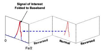
The effect of undersampling, as you probably expected, is that the IF signal is folded down to the first page. This is really an automatic frequency translation, performed for free by the sampling process.
