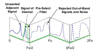
For the baseband **pre-select** sampling mode, we need to use a bandpass filter with the frequency response shown in green.
