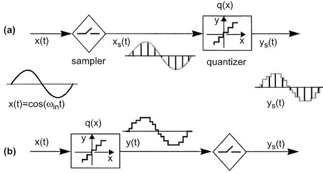
Fig. 1. ADC modeled as (a) a sampler preceding a quantizer or (b) a sampler following a quantizer [17].
