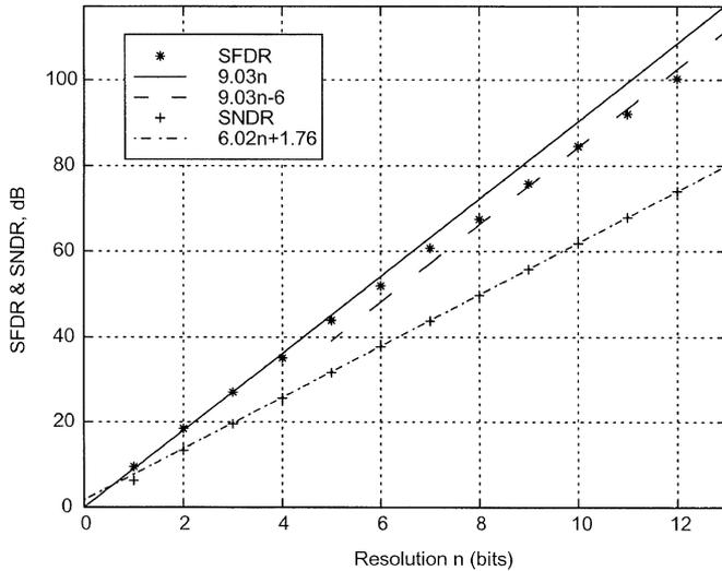
Fig. 3. SFDR and SNDR versus resolution  $n$  for ideal quantizers digitizing an FS sinusoid, simulated in MATLAB.
