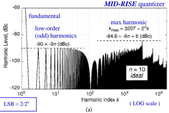
Fig. 1. Spectra of quantized sine wave. (a) Ideal 10-bit quantizer.
