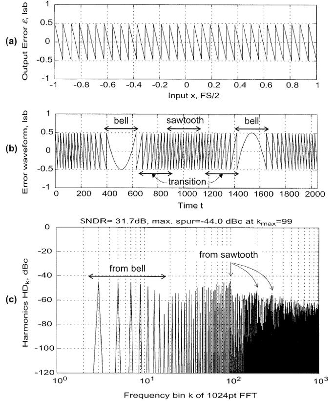
Fig. 2. A 5-bit quantizer ( $n = 5$ ) digitizing a  $FS$  sinewave, simulated in MATLAB. (a) Sawtooth input-output error characteristic. (b) Error waveform. (c) Output spectrum.
