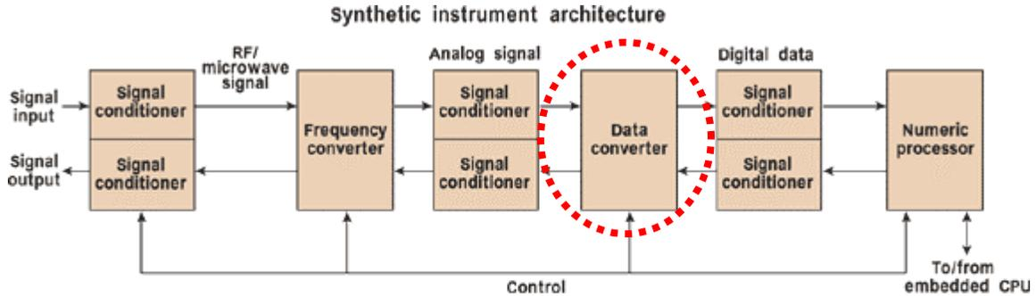
A basic SI system consists of a high-speed ADC and DAC at the core of the measurement system, as well as signal conditioning and up-converters and down-converters. Some would recognize this concept as "software radio."
