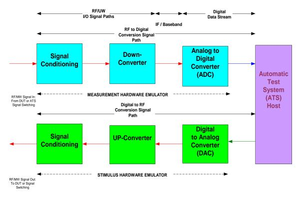
Fig. 1 Synthetic Instrument Based ATS: Notional Block Diagram
