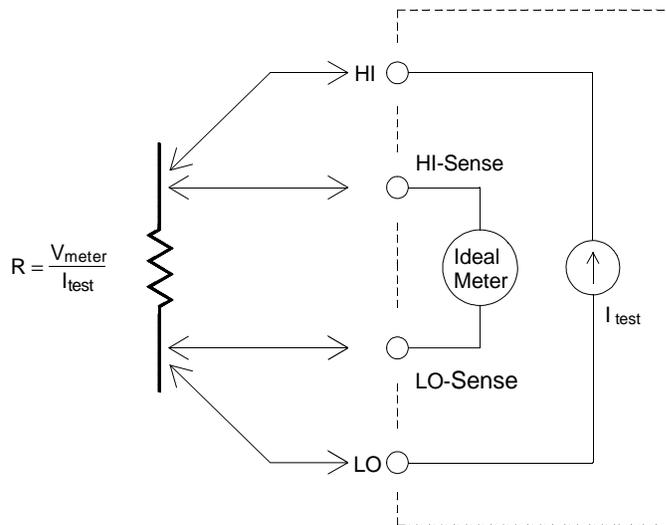
**Removing Test Lead Resistance Errors****Removing Test Lead Resistance Errors**
