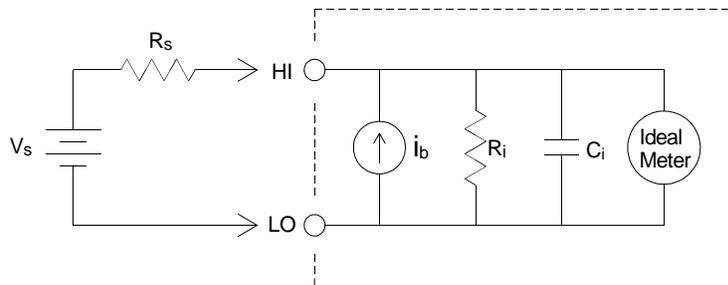
$i_b$  = multimeter bias current
