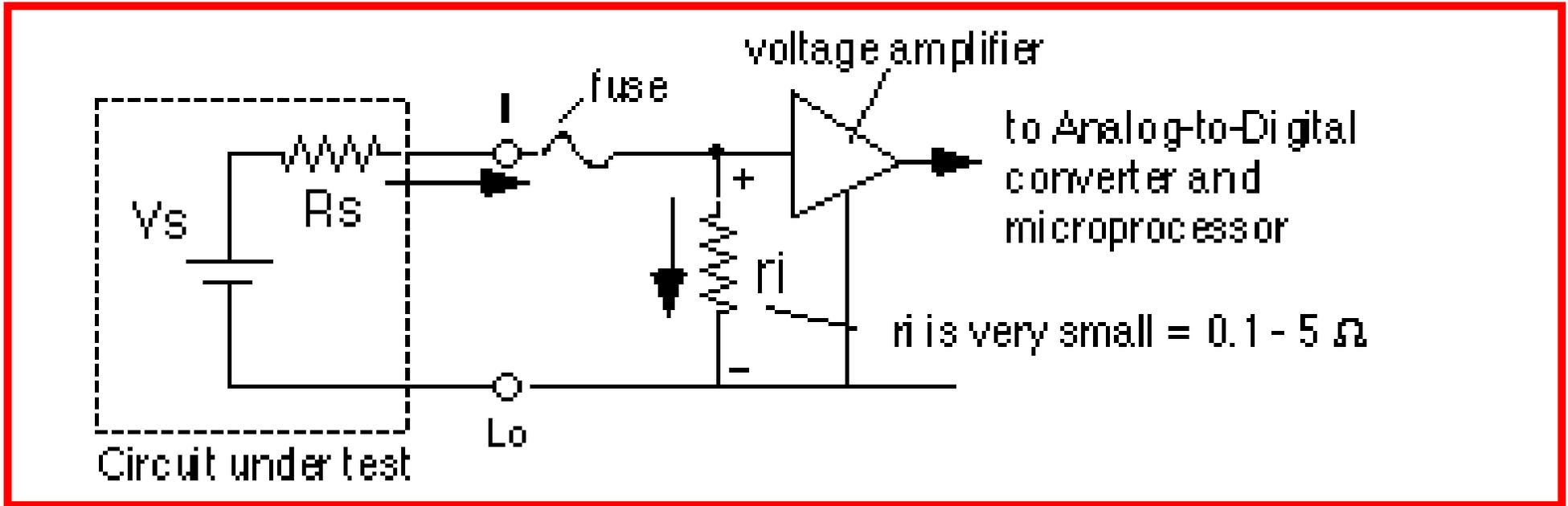
Principle of DC current measurement.
