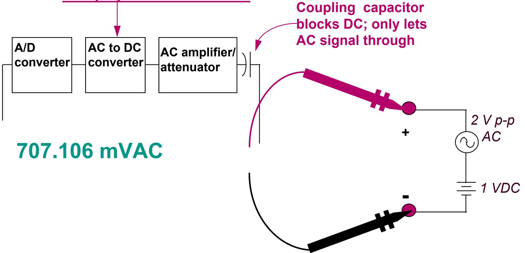
Note: measurement indicates only the AC portion of signal
