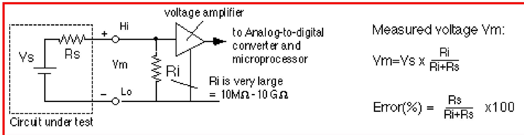
Schematic of the DMM as a DC voltage meter.
