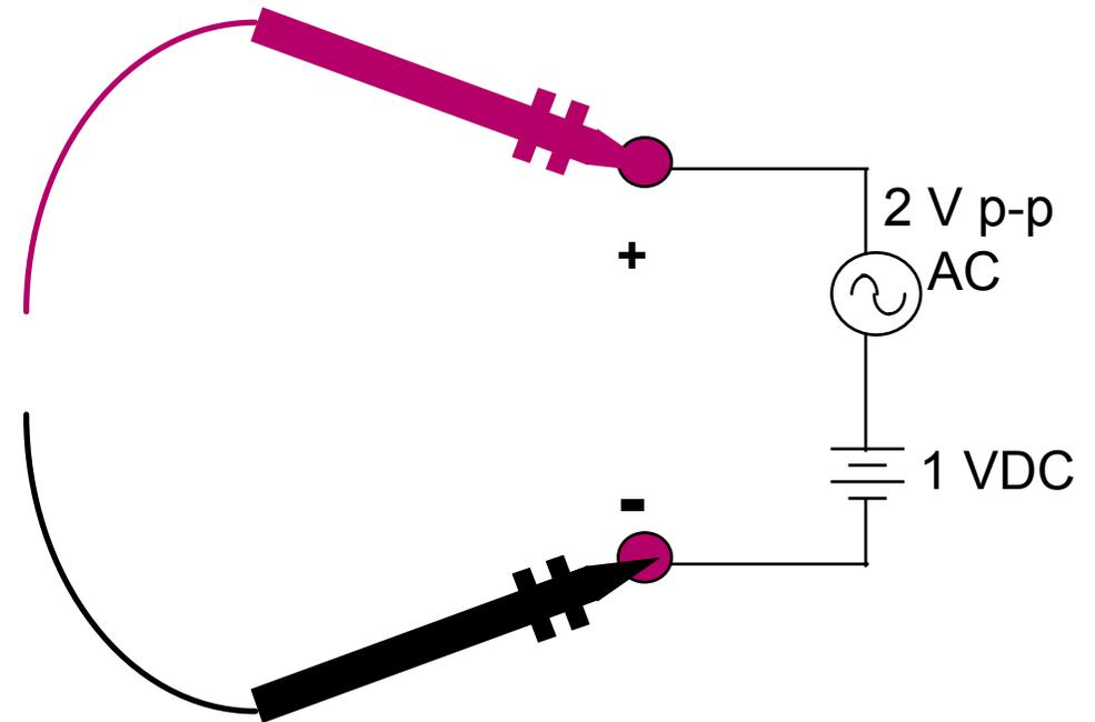
Note: measurement indicates only DC portion of signal
