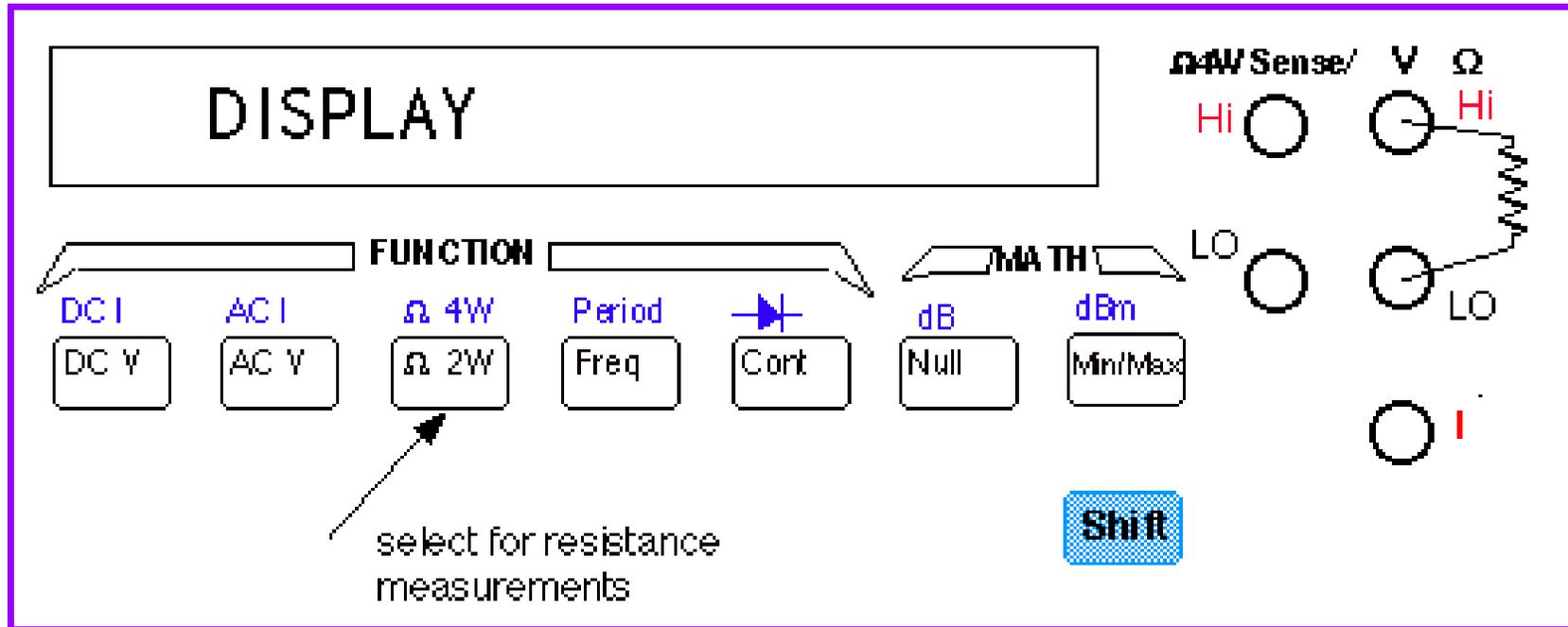
Function buttons to select resistance, voltage, current or frequency
