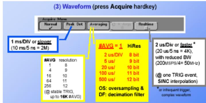
At the faster sweep speeds, the **running** display is built from many individual triggers. If you press the **Stop** key, and *pan and zoom* through the waveform by using the Horizontal and Vertical knobs, *only the last trigger's* acquisition will be displayed.
