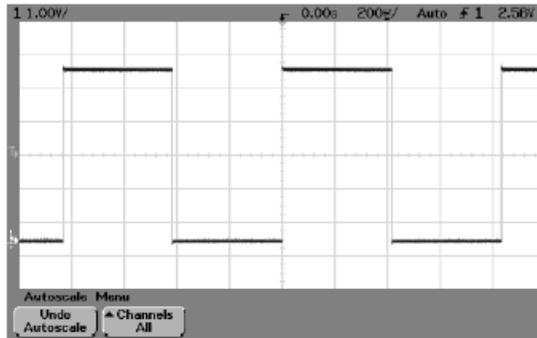
Autoscale finds, turns **ON**, and scales any channel with a **repetitive** waveform with a frequency of at least 50 Hz, a duty cycle greater than 0.5%, and an amplitude of at least 10 mV peak-to-peak.
