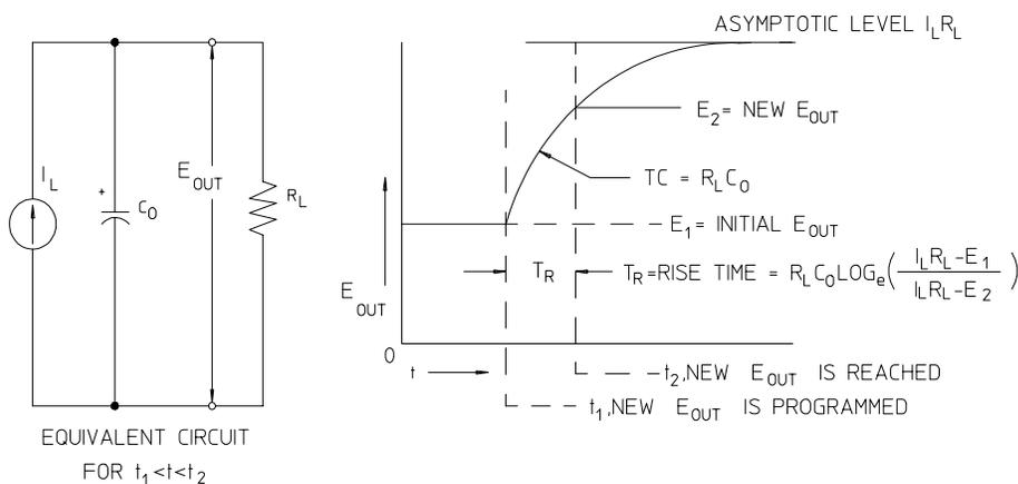
**Figure 7-7. Speed of Response - Programming Up (Full Load)**
