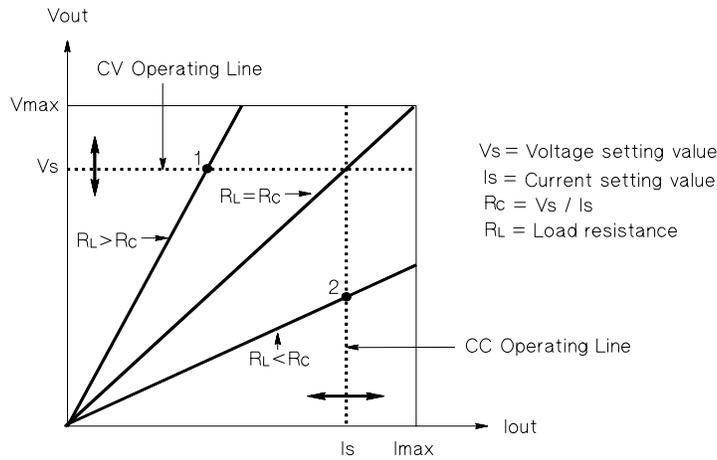
Figure 7-5. Output Characteristics
