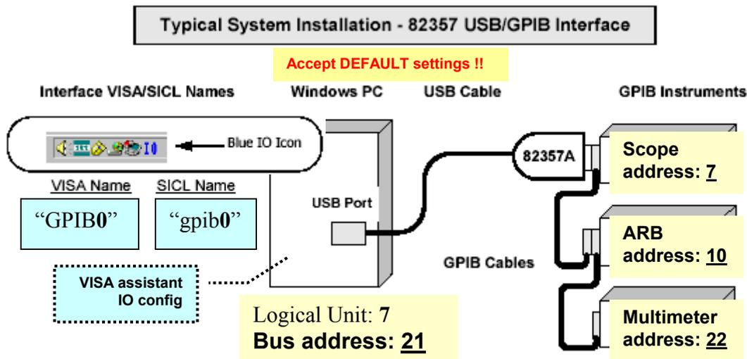
After the 82357A is successfully installed and configured, the interface should act as a **transparent** interface for programming GPIB instruments.
