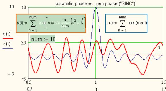
Note: The low-crest-factor signal resembles a chirped FM signal with monotonically increasing instantaneous frequency (LIN sweep, swept sine)
