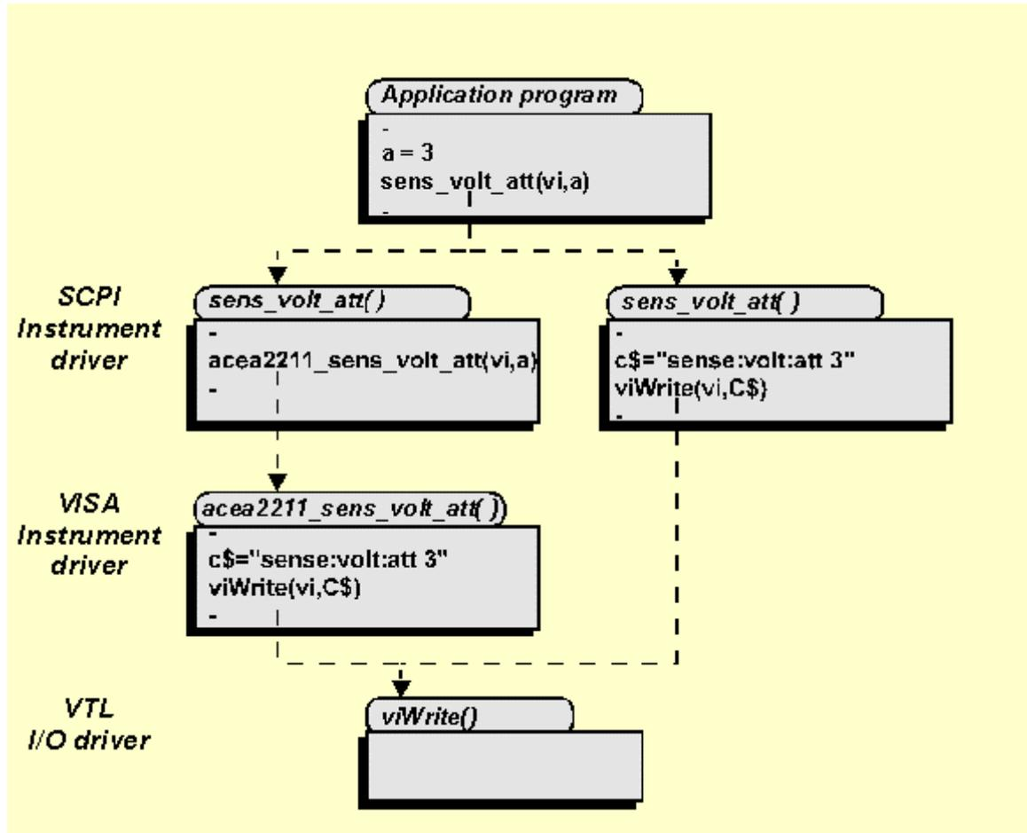
Figure 4. Vendor independent Instrument driver structure
