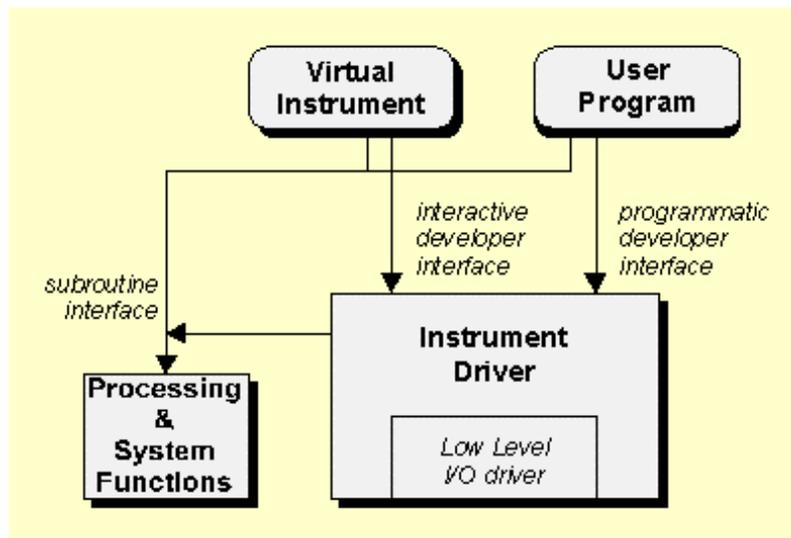
Figure 2. Application layer functionality
