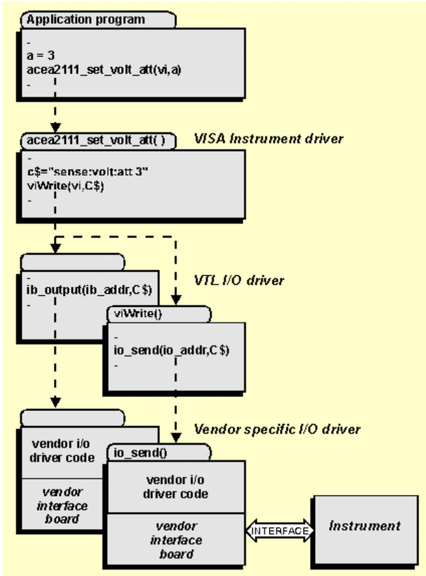
**Figure 3.** Survey of the structure of an instrument driver
