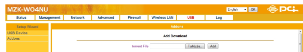
Figure 2. The management page of the Planex MZK-W04NU wireless router contains an image in the upper left corner with a unique file name identifying the device.
