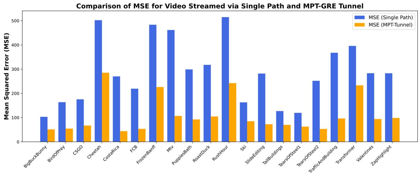
**Figure 6.** MSE comparison for different videos streaming via the single path and MPT-GRE tunnel.
