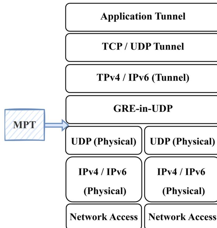
**Figure 1.** The conceptual architecture of MPT-GRE [17].
