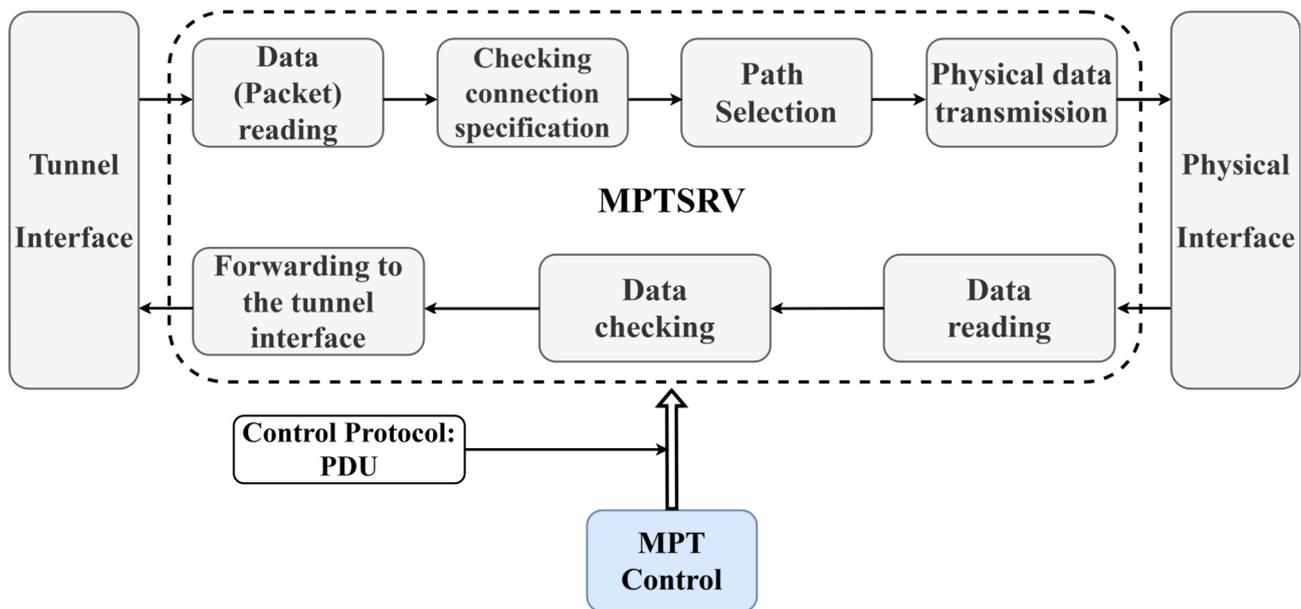
Figure 2. The theoretical process of the MPT-GRE mechanism [17].
