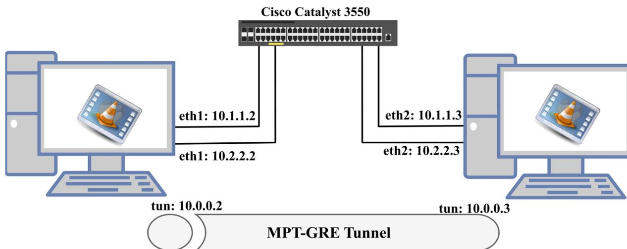
**Figure 4.** MPT-GRE multipath network topology of real-time 4K video streaming.
