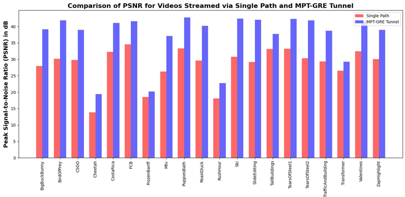
Figure 7. PSNR comparison for different videos streaming via the single path and MPT-GRE tunnel.
