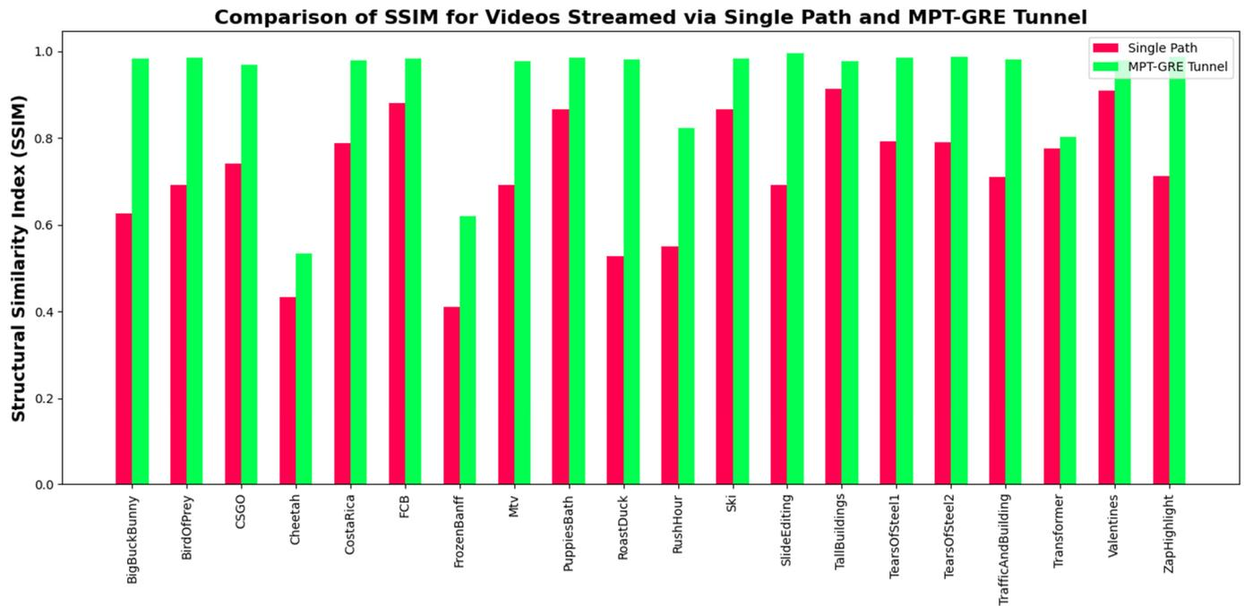
**Figure 5.** SSIM comparison for different videos streaming via the single path and MPT-GRE tunnel.
